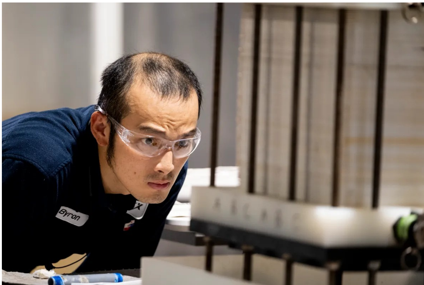
EnergyX Electrolysis Engineer Byron Tseng watches over the membrane stack during the bipolar electrolysis process of the direct lithium extract process. Michael Cavazos for The Texas Tribune
